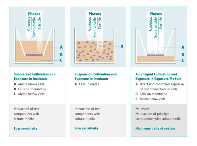
The exposure of mammalian cells or tissues to airborne substances is frequently performed under submerged conditions. In doing so, the test substances are dosed into the culture media. This procedure results in an undesired interaction of the formerly airborne substances with the media, causing limitations for authentic analysis.
