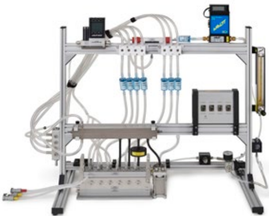
Rack with Dosimetry Module and Photometer connected to Exposure Module.
