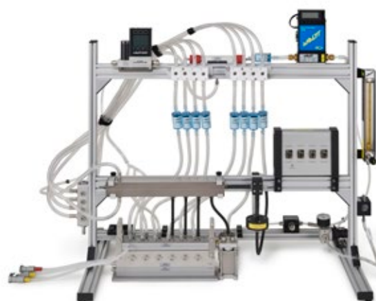
Rack with Dosimetry Module and Photometer connected to the main aerosol flow.
